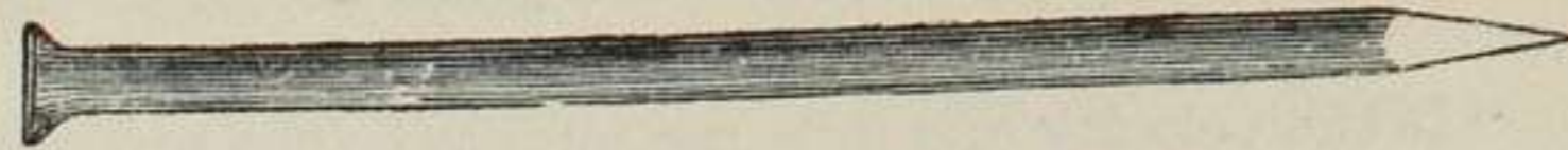
Fig. 236.—Round Wire Nail
