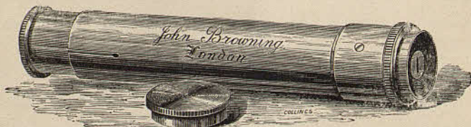
FIG. 29.—Direct Vision Spectroscope.
